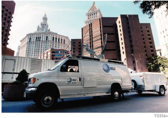
Figure 5.3-1: An Emergency Communication Vehicle (ECV) at the World Trade Center Police command center in September 2001. ECVs bring voice/data service up within minutes of arriving on scene.
