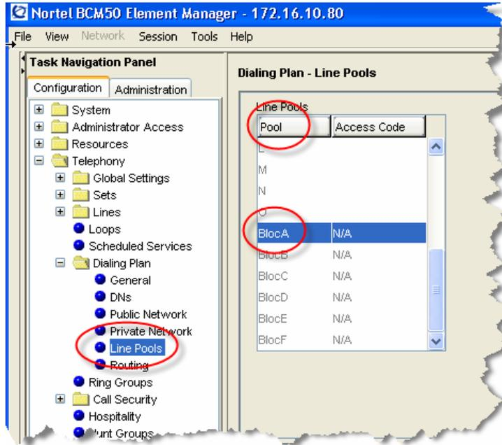
Figure 5: Assigning Line Pool to IP Trunks
