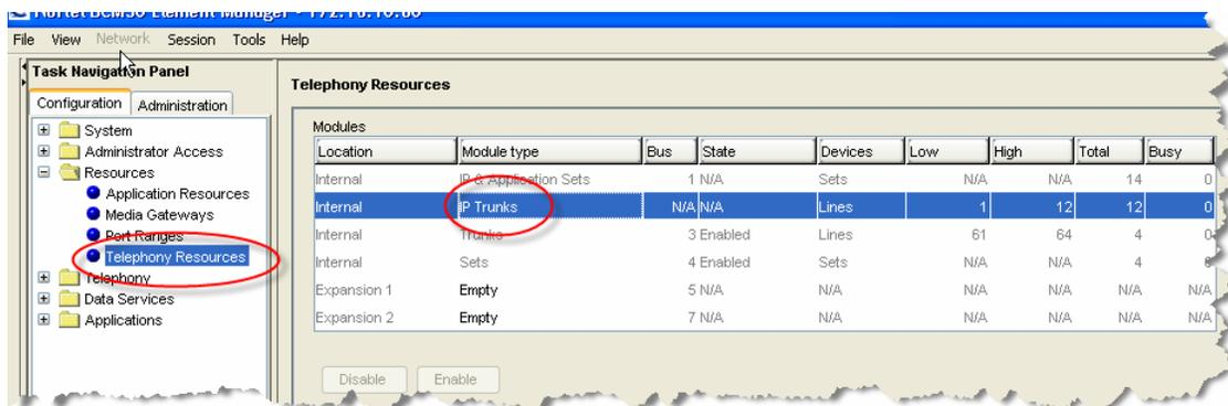
Figure 9: Selecting IP Trunk Module for H.323 Gateway
