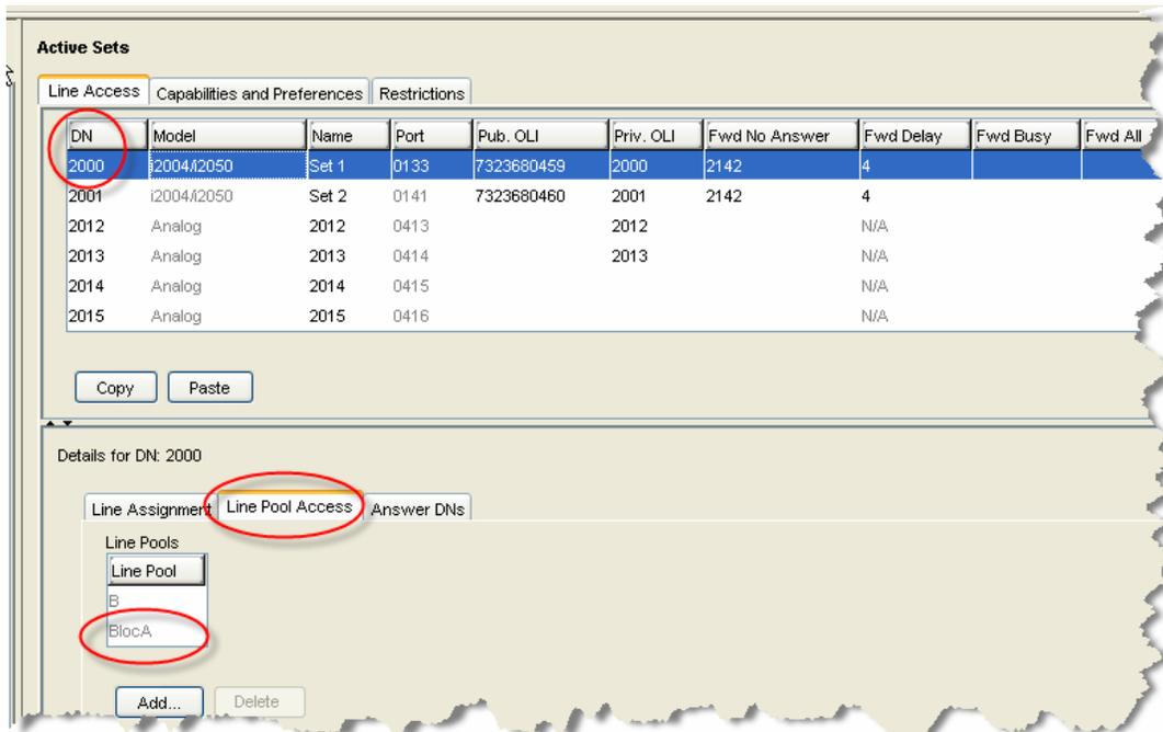
Figure 16: Assign Line Pool to IP Sets
