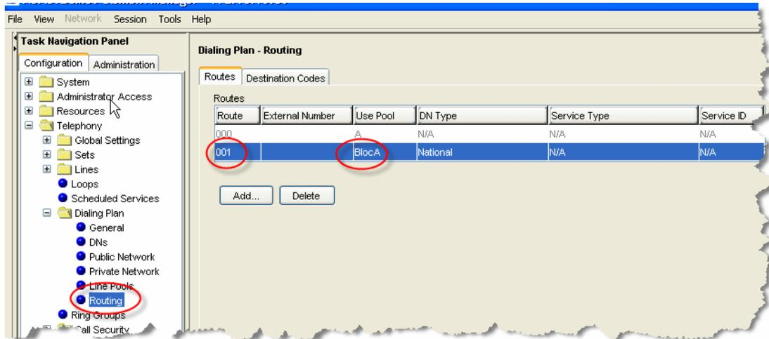
Figure 7: Assigning a Route for IP Trunks
