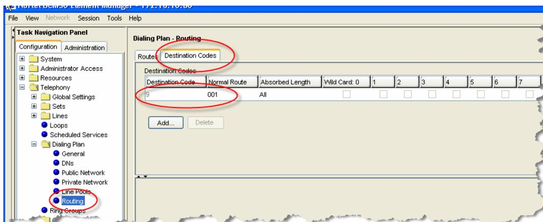
Figure 8: Assign Code to Access IP Trunk Routes
