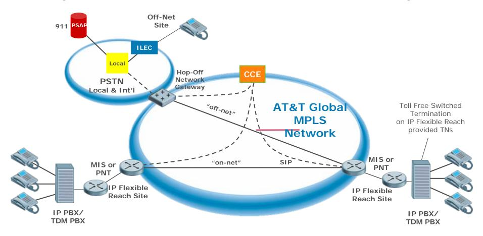
**Note:** IP Flexible Reach calling plans B & C options support TDM digital PBX or IP PBX configurations and is capable of supporting Toll Free Switched termination such as AT&T Readyline service. The Network diagram above depicts all configurations for illustrative purposes.
