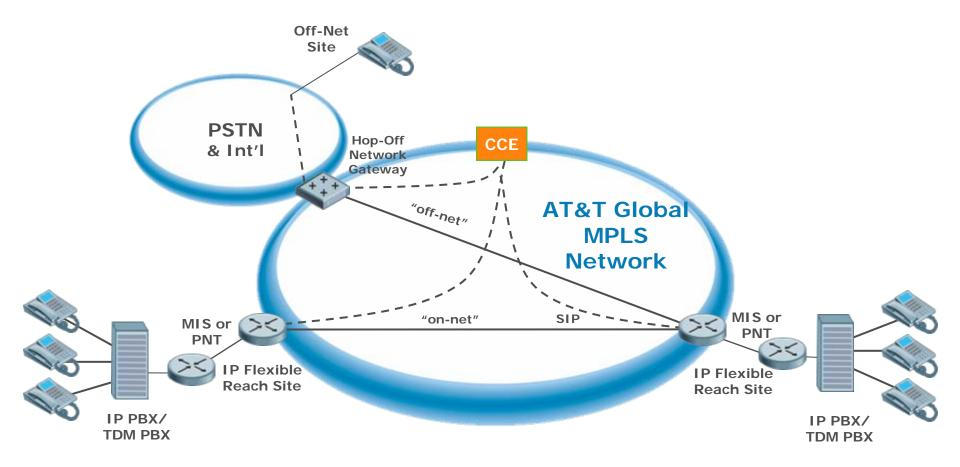
**Note:** IP Flexible Reach calling plan A options support TDM digital PBX or IP PBX configurations. The Network diagram above depicts both configurations for illustrative purposes. TDM PBX configurations require a voice card.
