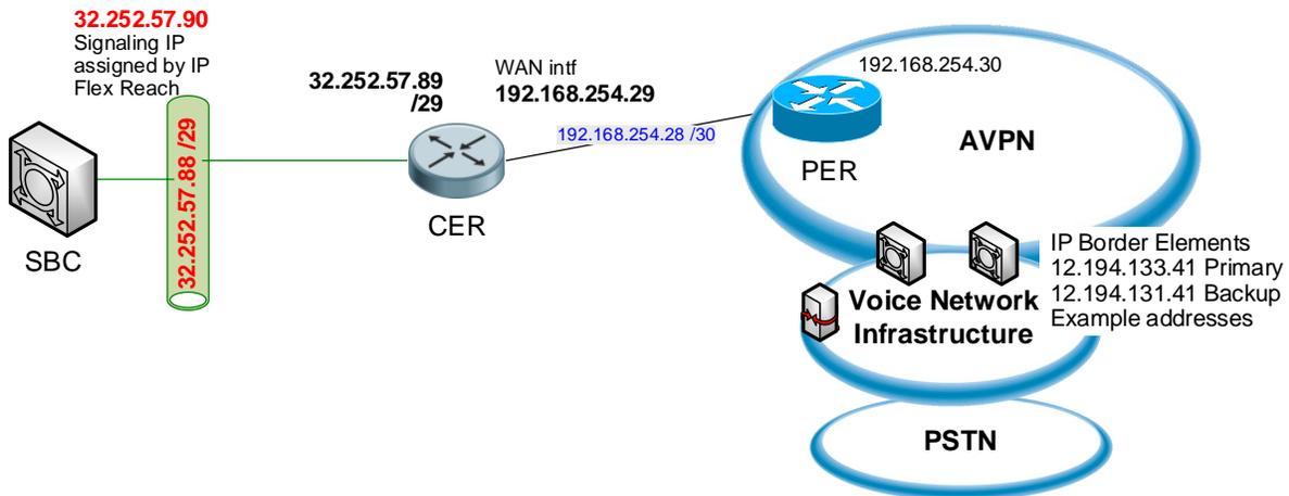
Figure 2 Alternate LAN Signaling Addressing
