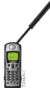
Figure 1.7.6.c-4: Iridium's Motorola 9500 Handset. Iridium constellation is typically accessed by low-cost handheld devices that give Agency personnel the freedom to roam anywhere on earth and stay in touch.
