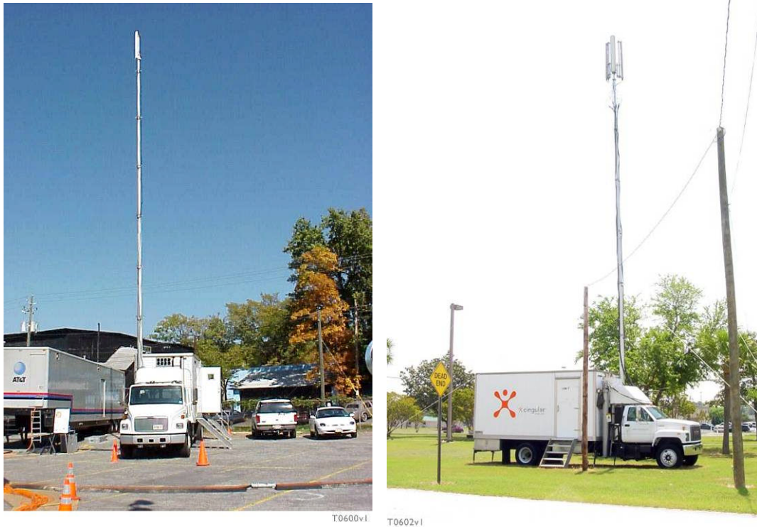
Figure 1.7.1.4-3: Cell-on-Wheels. Cingular operates many Cell-on-Wheels that are capable of quickly restoring communications to an area stricken by disaster.
